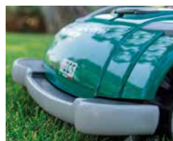
Bara de protectie si senzor de obstacol Bumper and obstacle sensor
